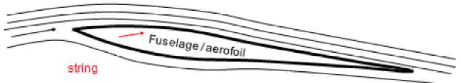
Viewed from above the fuselage is in the shape of a symmetrical wing. It is an aerofoil viewed at any angle. Therefore if we apply a positive angle of attack to it, it will produce lift off the fuselage, which actually has about two thirds the surface area of a wing (but sadly not that efficient!)
