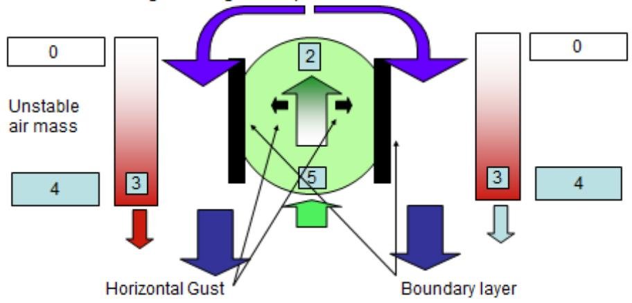
Formation of column thermals, in an unstable layer from a constant heat source. Notice how the volume of the thermal is increases vertically by extending down, not
