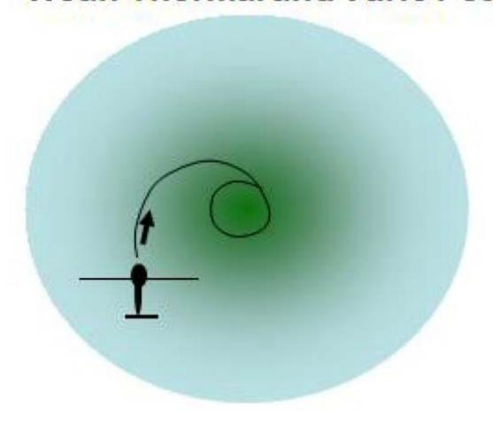
Right Wing Lifts therefore turn right with increasing bank (keep tightening the turn) until a maximum turn is achieved.
