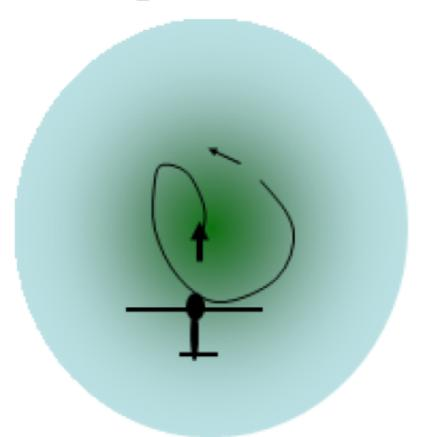
When the vario has been giving an increasing climb for 3 seconds turn using full aileron and rudder—it does not matter which way you turn—so long as you turn! You anchor the wing tip at that point.
